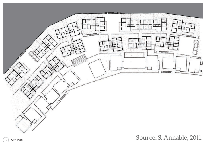
Figure 4: Plan of student-proposed neighborhood with public spaces, housing, and retaining walls. Integrated with the retaining walls, the first phase of development, are public amenities such as stairs, restrooms, and fresh water.
